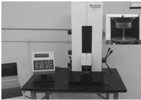
Fig. 3. Apparatus measurement spring coefficient constant (force changes in terms of length)
